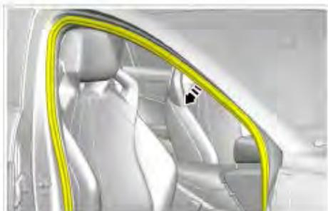
3. Carefully pry out the right A-pillar upper shield assembly with a plastic pry plate.
