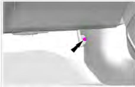
1. Remove 1 plastic nut from the right A-pillar lower shield assembly.
