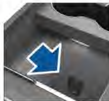
Figure 2 – LV power socket 2025+ Model Y
