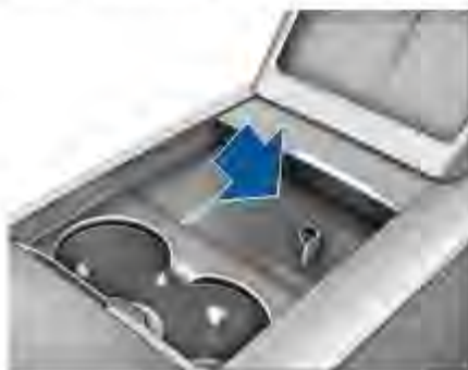
Figure 1 – LV power socket 2024+ Model 3
