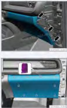
5. Disconnect the 9 fixing clips connecting the right lower trim panel assembly to the instrument panel body assembly, and remove the right lower trim panel assembly.
