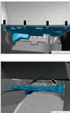
3. Disconnect 1 wiring harness connector connecting the ECALL speaker to the instrument panel wiring harness, and remove the right lower acoustic panel assembly with ECALL speaker.
