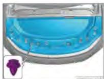
4. Disengage the 9 fixing clips of the front compartment trim panel assembly with a plastic pry plate, and remove the front compartment trim panel assembly.
