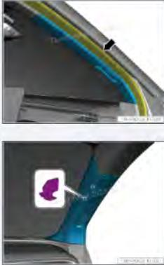
3. Disengage the 2 metal clips connecting the right A-pillar upper trim panel assembly to the vehicle body, and remove the right A-pillar upper trim panel assembly.
